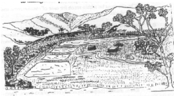
Fig. 2: Small valleys with gentle slope have excellent potential for pond construction
